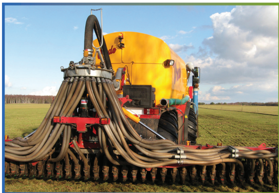
European-style disk injector pulled by a tanker with crab steering to avoid compaction
